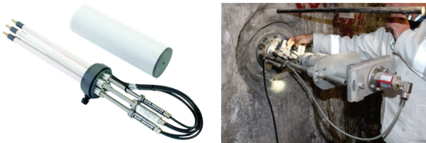
Figure 3.15: Rod Extensometer and its installation [16].
